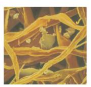
Advanced techniques and huge laboratory resources are needed to produce a filter paper with exactly the right pore structure. The photo shows a Volvo genuine filter paper magnified 100 times.
